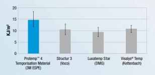
In a test measuring material toughness, Protemp<sup>™</sup> 4 Temporisation Material showed greater resistance to fracture than other tested temporisation materials. Source: Schwarz et. al., AADR 2014 accepted
