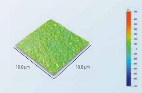
Surface topology of Protemp" 4 Material after removing the inhibition layer with alcohol and no further polishing. Source: 3M ESPE internal data – Atomic Force Microscopy (AFM) images by 3M Corporate Research Analytical Laboratory – (CRAL)
